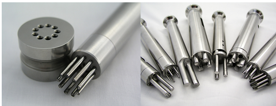
FIGURE 6.4 Mini-tablet tooling: punch and die combination (left); different designs exist for mini-tablet multitip tooling, such as multiple part cap-and-pin design and solid multitip design (right). In a monoblock design, all tips are machined from one piece of stainless steel. Mini-tablet tooling can also be produced with different shapes and varying number of tips. The upper punch for mini-tablet tooling is keyed to maintain its rotational orientation. Pictures are courtesy of Natoli.
